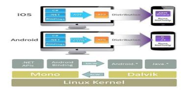
Fig.9. The process of compiling native Xamarin assemblies
